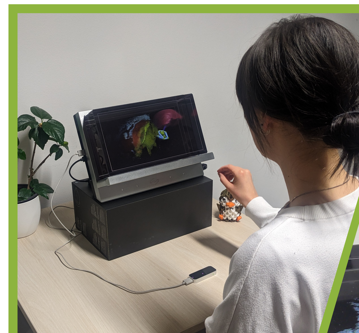
Fig. 1: A user interacting with our proposed system. It consists of a stereoscopic display and a hand tracking device.
