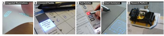
Figure 1. Our ILLUMIPAPER research platform (E) provides paper-integrated visual feedback without losing the sensory richness and flexibility of paper (A) and supports several applications including educational grid puzzles (B), interactive tool palettes (C) or even math exercise sheets (D).
