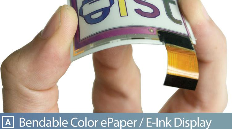
We build on a *bendable* active-matrix electrophoretic display (EPD) from Plastic Logic with *AdvancedColor* (ACeP) ePaper technology providing four color pig-
