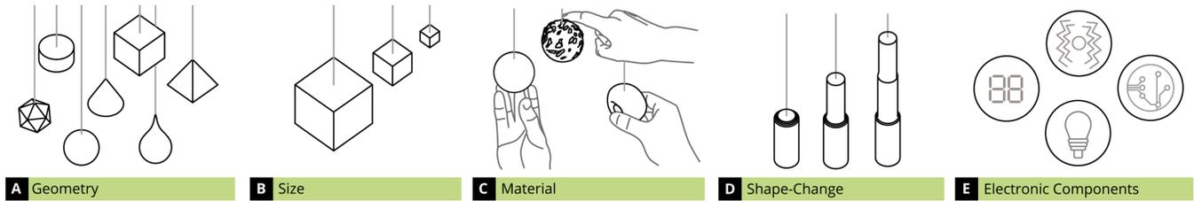
**Figure 2: Display elements can differ in their geometry (A), size (B) as well as material, texture, and other haptic properties (C). In addition, shape-changing capabilities (D) as well as further electronic components (E) (e.g., touch input, vibrotactile feedback, displays, and illumination) can be integrated.**
