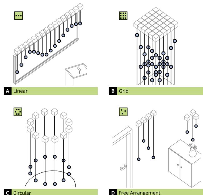
**Figure 3: Physical assemblies of actuated elements come in different arrangements and layouts. For instance, elements can be placed in a linear order (A), arranged along a regular grid (B) or a circular path (C), or positioned where they are needed (D).**
