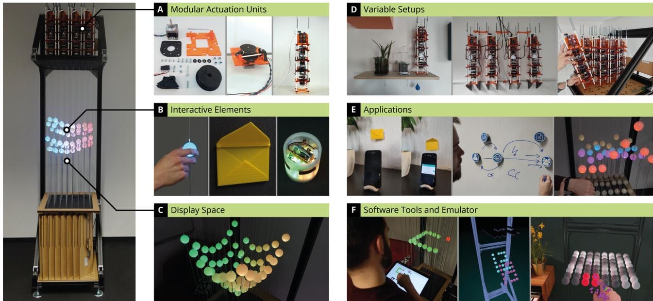
Figure 1: STRAIDE comprises modular actuation units (A) that actuate a variety of passive or (inter)active elements (B) to create casual visualizations in mid-air (C). The actuators are arranged in different setups (D) to enable situated applications with an increasing number of elements (E) ranging from ambient notifications to visual storytelling to casual information visualization. A set of supplementary software tools (F) reduces the effort of application development.
