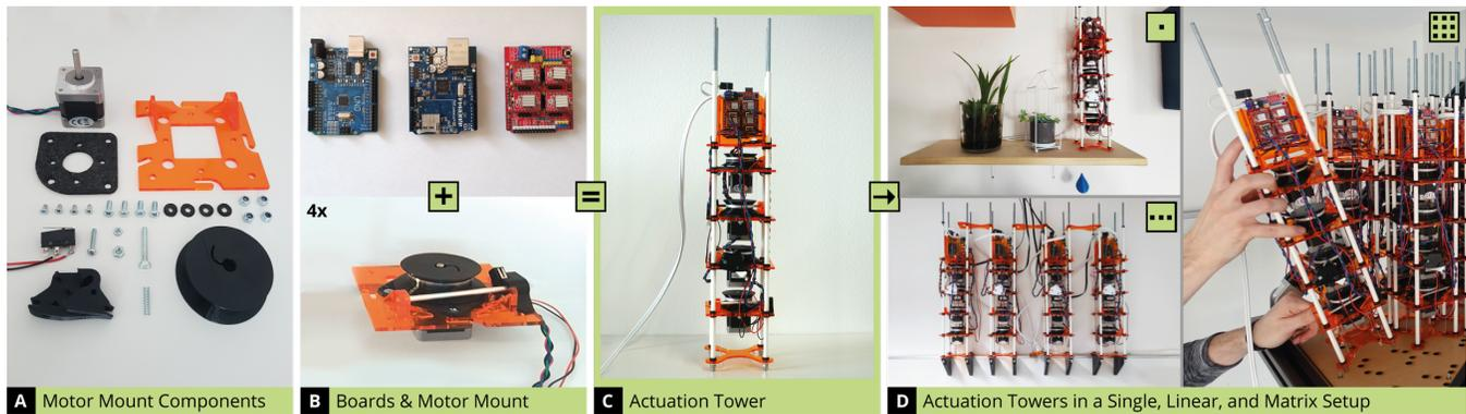
**Figure 8: STRAIDE’s actuation is based on stepper motors in custom laser-cut mounts (A) that are assembled and combined with a stack of microcontroller boards (B) to form self-contained actuation towers (C). These are employed in different setups (D), for instance in a Single, Linear, or Matrix Setup.**
