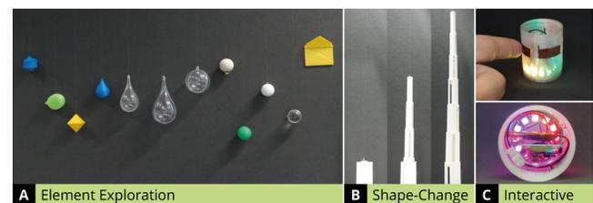
**Figure 6: In our technical exploration we evaluated a variety of elements (A, left to right) with different shapes, sizes, materials, shape-changing capabilities (B) as well as interactive elements (C). The latter example uses a WiFi-capable micro-controller powered by a battery to control LEDs and detect touch.**
