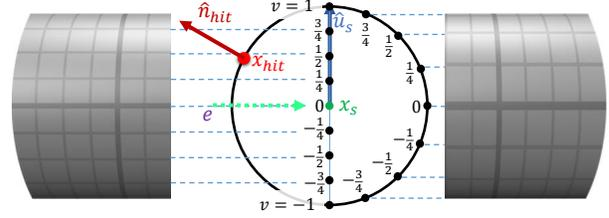
Fig. 6. Illustration of the two strategies to parameterize tube surface around center curve. Left: equidistant in screen space; right: arc length parameterization.
