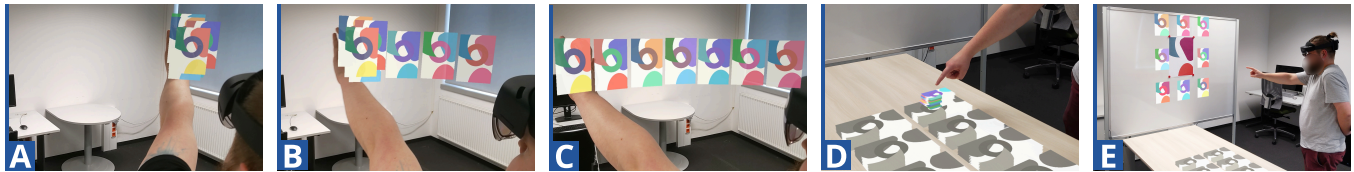
Figure 16: To compare graphic design variations: (A-C) transforming a stack into a row by brushing the resulting layout; (D) tapping to snap selected files onto the fingertip; (E) drawing to arrange a grid layout around the physical poster.
