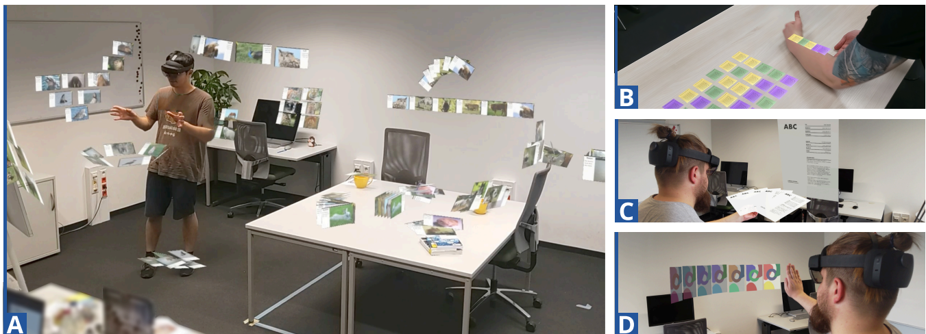
Figure 1: (A) We conducted a study where participants proposed interaction techniques for arranging AR documents. Based on the findings, we introduce a design space, derive design implications, and illustrate use cases with a rapid prototyping system. These use cases include (B) affinity diagramming (classifying and clustering sticky notes), (C) document management (fanning out documents and enlarging one), and (D) graphic design iteration (brushing a row layout to compare variants).
