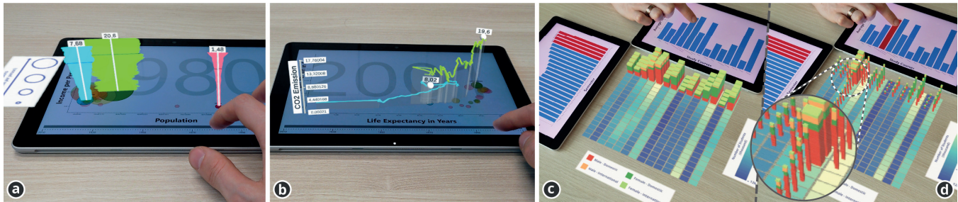
Figure 7: Showing 3D visualizations above and between devices: (a) Scatterplot extended with 3D glyphs; (b) Another scatterplot superimposed with 3D trajectories based on the position (x, y, z) over time; (c) AR heatmap and stacked bars resulting from a combination of visualizations and devices; (d) Since rows and columns are selected, individual cells and stacked bars at the intersection are highlighted.
