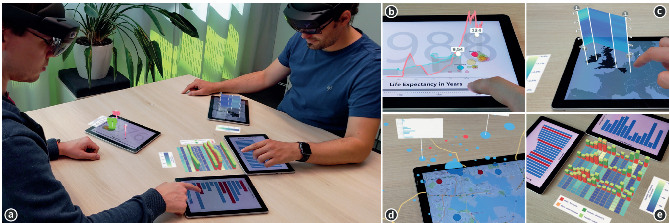
Figure 1: Data visualization using mobile devices and Augmented Reality head-mounted displays: (a) Envisioned usage scenario; (b) 2D scatterplot extended with superimposed 3D trajectories/paths; (c) 3D wall visualization in AR aligned with the mobile device; (d) Use of AR for seamless display extension around a geographic map; (e) Combining visualizations with an AR view between the devices.
