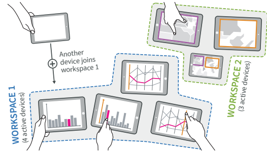
Figure 2: Workspaces control view (device) coordinations. While workspace 1 illustrates linked brushing , workspace 2 shows a overview & detail setting.
