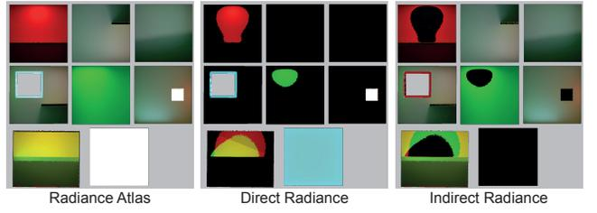
Figure 5: The radiance atlas (left) is split in direct radiance (middle) and indirect radiance (right). Note that the direct radiance atlas contains both the light sources and bright indirect regions. The separation is computed per color channel to allow sources in monochrome regions that would have a low gray scale brightness.
