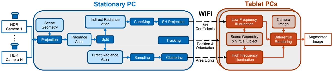
Figure 3: The whole pipeline for distributed illumination.
