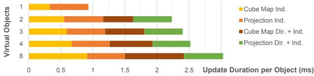
Figure 11: Timings for updating the indirect light coefficients per object. Measured in the CORNELL SCENE with multiple virtual BUNNIES.
