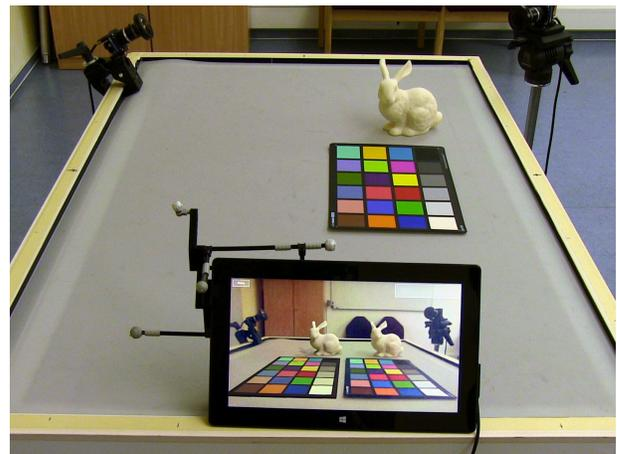
Figure 1: The tablet camera shows the real world, augmented by virtual objects with consistent illumination, displayed at 27 fps. By using a tracked device, the user can move the tablet freely in the augmented real world.
