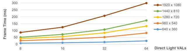
Figure 12: Influence of the G-Buffer resolution on the frame time. Timings measured for augmenting the CORNELL SCENE with the virtual BUNNY.
