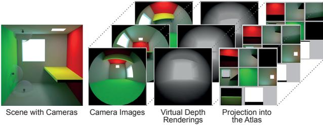
Figure 4: Acquiring the radiance atlas for a simple synthetic scene with three HDR cameras (left). Each HDR camera records a fish-eye image of the scene. Additionally, a depth buffer is rendered for each camera using the reconstructed scene. Using the depth buffer for visibility tests, the camera image is then projected into the radiance atlas (right). Note that each camera has only a partial information of the total scene radiance.
