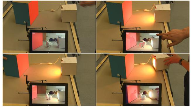
Figure 16: Moving tracked objects: Initial configuration (top left), user switches on the light and rotates the BUNNY at 27 fps (top right), red color bleeding disappears when the box is moved away (bottom left) and direct light changes after light movement (bottom right).
