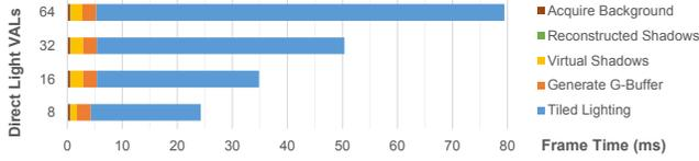
Figure 13: Timings with respect to the number of VALs measured for augmenting the CORNELL SCENE with the virtual BUNNY broken down and accumulated.
