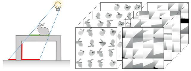
Figure 9: Two shadow maps per VAL are required to avoid double shadowing from virtual objects (dashed contour) in regions that are shadowed in the real environment.
