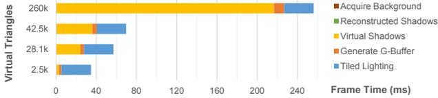
Figure 14: Timings with respect to vertex count measured for augmenting the CORNELL SCENE with different virtual models and 16 lights broken down and accumulated.
