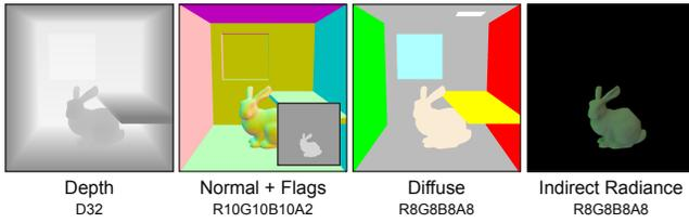
Figure 8: G-Buffer: an off-screen buffer containing geometry and material information of the reconstructed and virtual scene per pixel.
