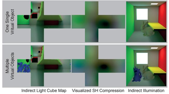
Figure 7: To estimate the indirect illumination of a virtual object, we first render a cube map with the indirect radiances from the object center (left). This is projected into the first nine SH basis functions (center) which allows a real-time illumination of a virtual object (right). The second row shows multiple virtual objects with mutual interreflections, like the blue color bleeding from DRAGON to BUNNY.
