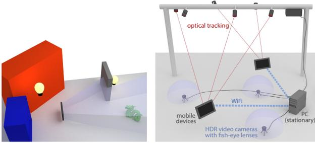
Figure 2: Left: The camera image of a mobile device does not see the important light sources required for a consistent illumination of a virtual object. Right: Our hardware setup.
