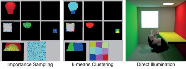
Figure 6: VAL extraction for direct light: Samples are placed on the direct radiance atlas (left). Using k-means clustering, these samples are grouped in  $M$  clusters (middle). Each texel is assigned to the closest cluster center. Integration over each cluster leads to  $M$  VALs that are used for direct illumination of a virtual object (right).
