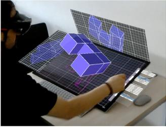
**Figure 2:** *DesignAR*: Orthographic views showing a 2D projection of the model, one of them is tilted for better visibility to the user.
