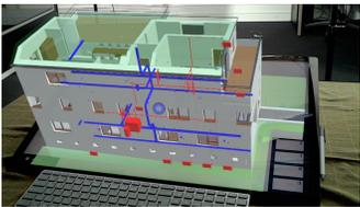
**Figure 6:** *ARchitecture*: 3D model of the building directly augmented and aligned with the technical drawing (with visible pipes for heating and electric cabling).
