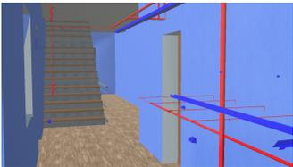
**Figure 7:** *ARchitecture*: Immersive first-person view through the portal next to the display (again with visible pipes for heating and electric cabling).
