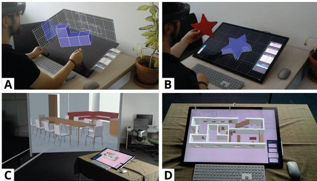
**Figure 1:** (A) Our immersive 3D modeling tool *DesignAR*, showing the model itself in the center, orthographic cutting views and offloaded menus. (B) 3D model created with pen input in *DesignAR* and based on a real-world object. (C) Our architectural design tool *ARchitecture*, showing the interactive surface, augmented view, and immersive portal view. (D) Close up of *ARchitecture*'s interactive surface with the augmented 3D representation.
