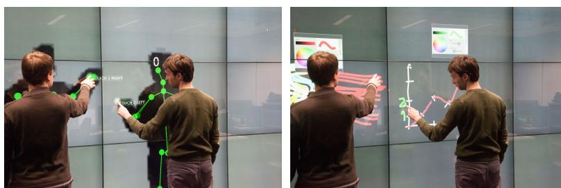
Figure 1: User-identification using an RGB+Depth camera. Left: Debug view showing user IDs. Right: Application context with user-specific brush settings (Zadow et al., 2016)
