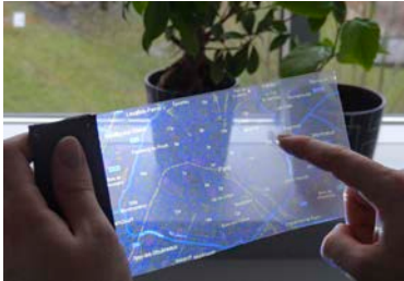
Figure 1. Non-interactive mockup, utilizing back-projection onto a transparent foil.
