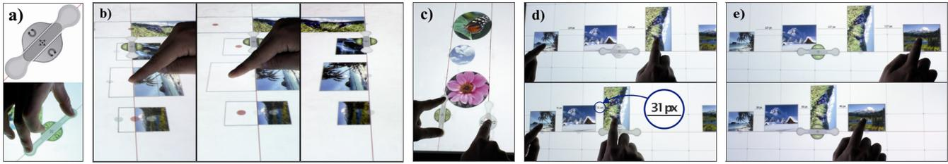
**Figure 2.** (a) Close-up of the handle, (b) changing the alignment by dragging an object across the guide (*all-mode* activated), (c) scaling objects by pushing two line guides together, (d) holding an object and dragging another one adjusts the spacing of objects in between, (e) *all-mode*: dragging one single object adjusts the spacing of other objects.
