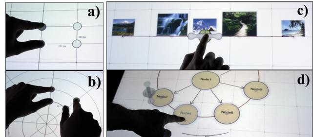
**Figure 1** *Interactive grids*: an orthogonal grid can be adjusted by multiple fingers (a) and seamlessly changed to a radial grid (b). *Multi-touch alignment guides*: objects are bound to shapes such as lines (c) or arcs (d). Alignment and spacing can be adjusted by touch input.
