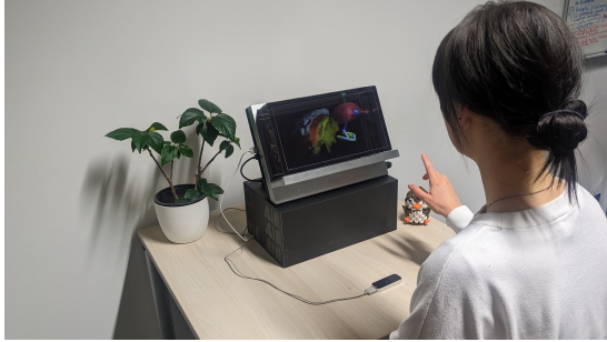
Figure 2: Our system [16] combines a stereoscopic display with hand tracking for a medical use case.
